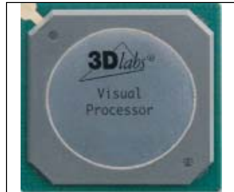
Figure 1 - P10 820-ball thermally-enhanced 37.5mm HSBGA package. (Not shown: P9 644-ball thermally-enhanced HSBGA in 31mm package.)
