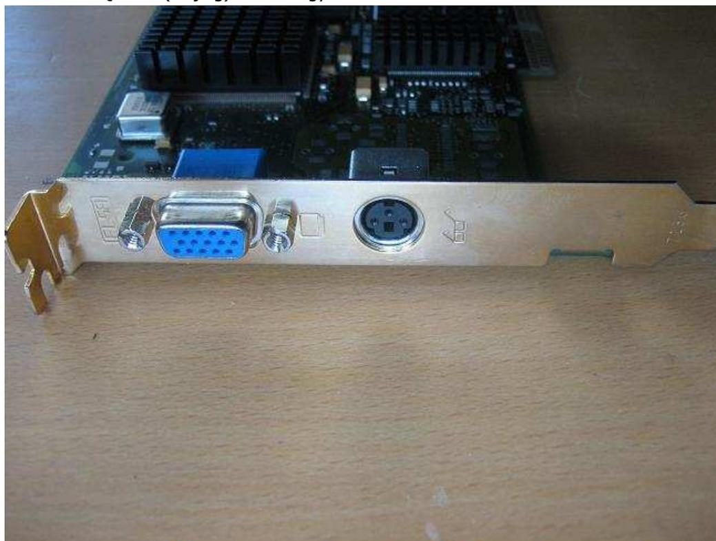
The graphics in addition to providing D-sub display output interface, and a 3-pin stereo glasses interface. Today's high-end professional graphics cards generally come with this interface, when I first saw this piece of card. In addition, I/O metal bracket, but after a gold-plated treatment.
