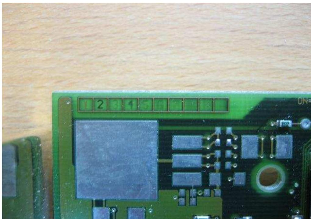
Gloria XXL card using 10-layer PCB board. Today, high-end gaming graphics using the 10-layer PCB is nothing new; but at the time, most of the mainstream gaming cards also 4-layer PCB, 6-layer PCB can only be seen in some high-end products, 10-layer PCB, but rather the cost of high.
