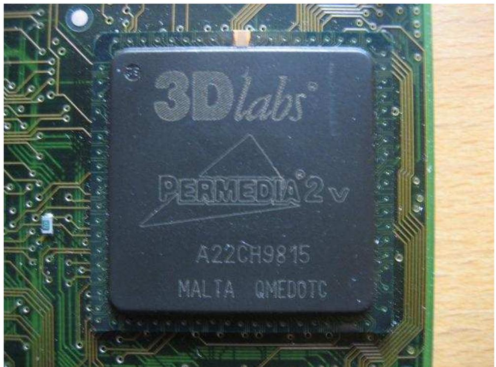
The only use of block graphics BGA package 3Dlabs PERMEDIA 2V chip, this card is only used in 2D the basic display. PERMEDIA 2 of the 2D performance is certainly outstanding
